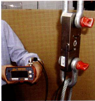
● 4. separate display with cable connection
