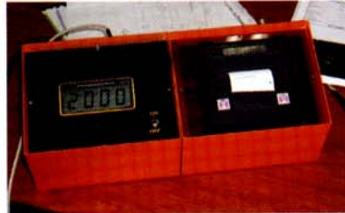
● 8. separate display with printer and radiotransmission
