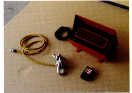
● 6. loadcell with separate display and remote control
